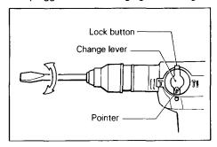
Depress the lock button and rotate the change lever so that the pointer points to the symbol. Then make sure that the bit is securely held in place by turning it slightly.
